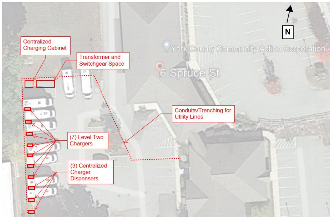
Figure 16 Conceptual Layout of Chargers at the 6 Spruce St. Facility (Source: Google Earth)
