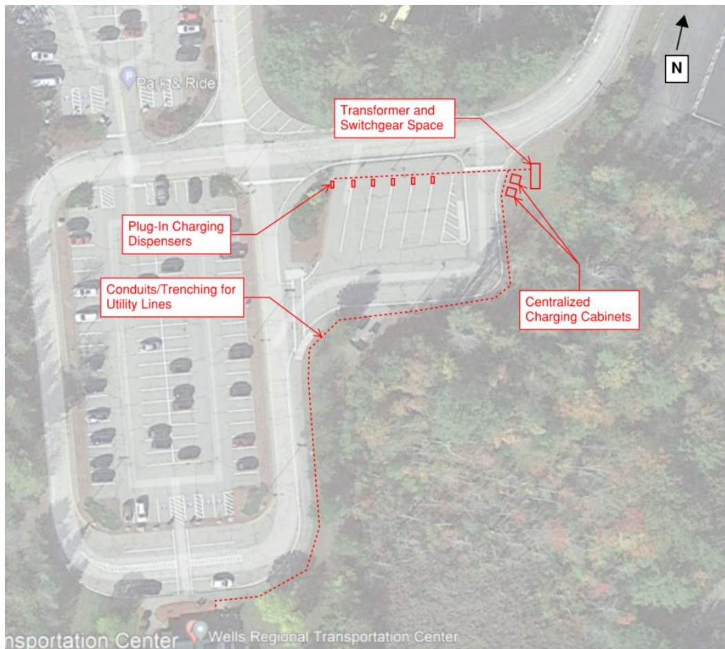
Figure 18 Conceptual Layout of Chargers at the Wells Regional Transportation Center (Source: Google Earth)
